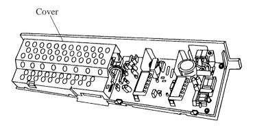
(8) Connect the IPC-2 option board connector and tighten the screw.
